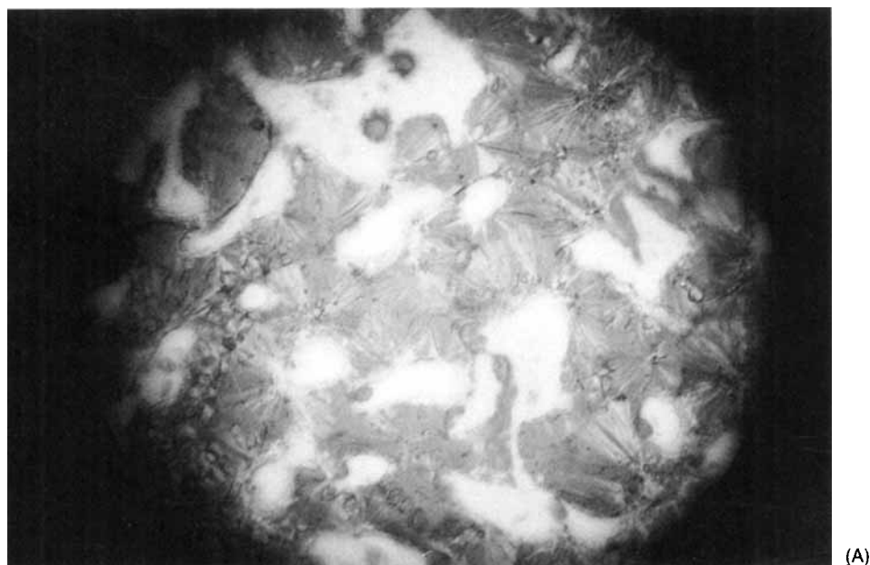
Figure 13 Polarized photomicrograph for PCL-CDA blends: (a) As-cast and (b) thermally treated 75/25 blend; as-cast 25/75 PCL-CDA blend.
